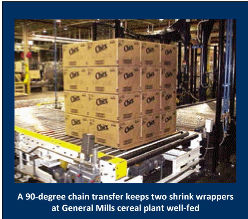
programmable logic controller directs a series of chain elevators running perpendicular to the conveyor path to lift the cube of cases clear of the rollers. The chains start turning, transferring the slip sheet and its stack of cases onto the bypass conveyor.
