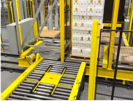
transfer car, each 40" x 48" GMA pallet is rotated 90° by an Alba lift and rotate CDLR conveyor. The half pallets are conveyed without needing rotation. The final step involves an electric turntable with a CDLR conveyor, rotating the pallets 90° before sending them down Weldon's integrated stretch wrapping line.
